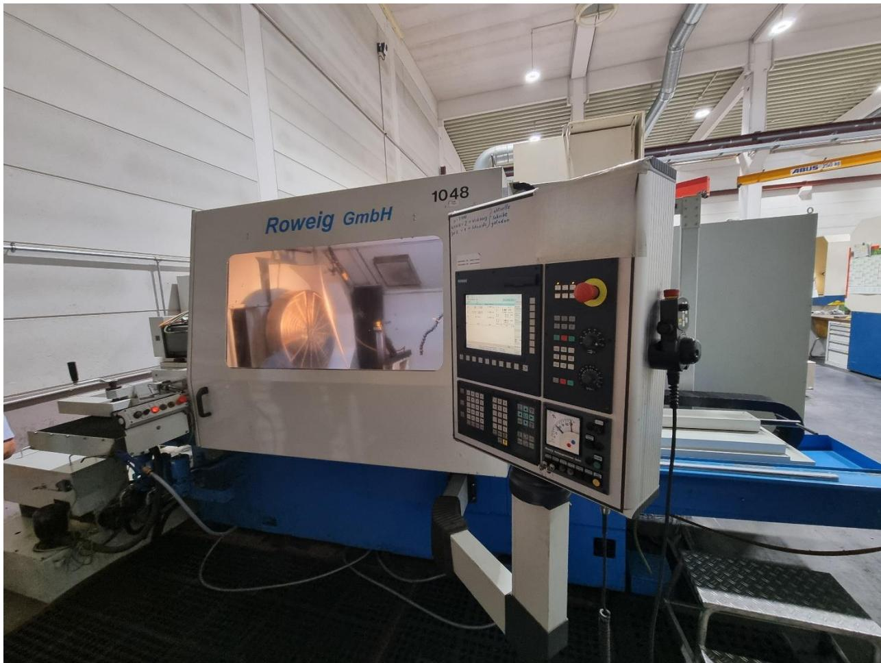
High-quality CNC internal cylindrical grinding machine for grinding cylindrical, conical, simple and stepped bores, short outside diameters and end faces
